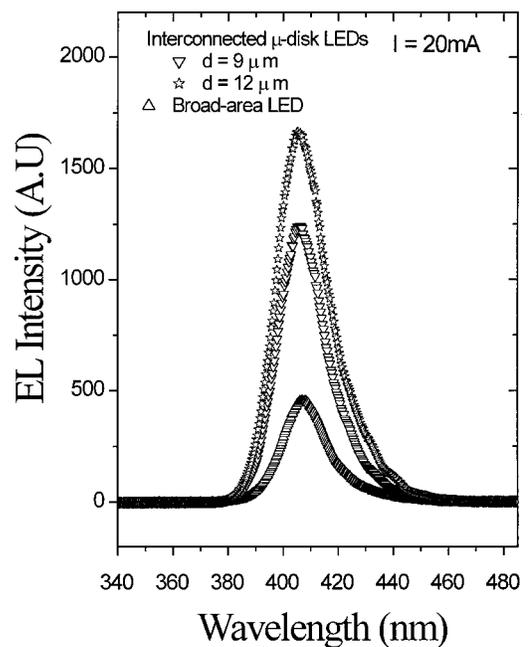
FIG. 3. Comparison of EL spectra of inter-connected  $\mu$ -disk LEDs with a conventional broad-area LED fabricated from the same InGaN/GaN QW wafer measured on the top surface of unpackaged chips at 20 mA.
