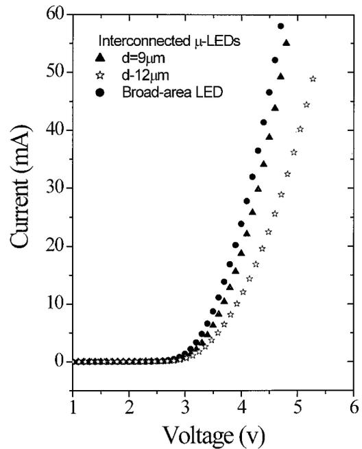
FIG. 2. Comparison of  $I$ - $V$  characteristics of inter-connected InGaN/GaN QW  $\mu$ -disk LEDs and a conventional broad-area LED fabricated from the same wafer measured on the top surface of unpackaged chips. Inter-connected  $\mu$ -disk LEDs comprise about 200  $\mu$  disks of diameters of 9 or  $12 \mu\text{m}$  and occupy the same device area as the conventional broad-area LED ( $300 \mu\text{m} \times 300 \mu\text{m}$ ).
