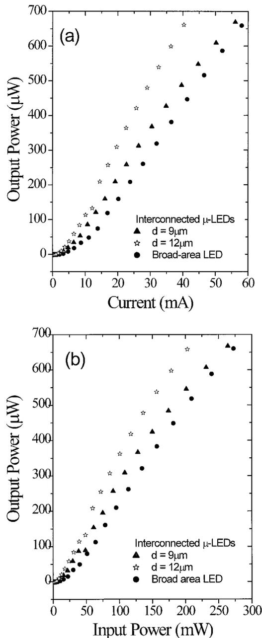
FIG. 4. Light output power vs (a) forward current and (b) input power for the interconnected  $\mu$ -disk LEDs and a conventional broad-area LED measured on the top surface ( $p$ -type GaN side) on unpackaged chips. Actual total output powers of these LEDs should be much higher than the measured values shown here since most of the light emission was not collected from these unpackaged chips.
