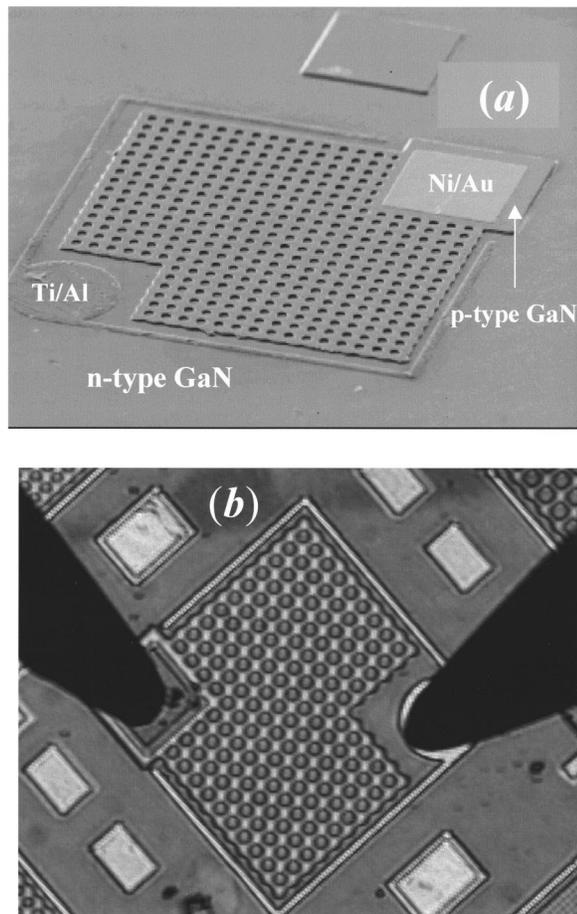
FIG. 1. (a) SEM and (b) optical microscope images of one of our inter-connected  $\mu$ -disk LEDs fabricated from InGaN/GaN QW structures. As illustrated in these images, about 200  $\mu$  disks are interconnected and fit into an area of  $300 \mu\text{m} \times 300 \mu\text{m}$ .
